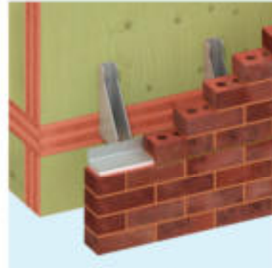
M8 x 100mm washer head SPAX screws should only be fixed into the edge of CLT panels. Heel screws should be fixed up into the middle of the CLT panel (not into the joints).
