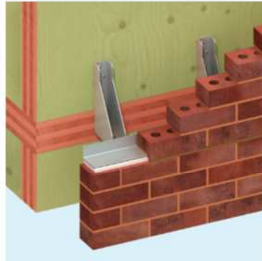
M8 x 100mm washer head SPAX screws should only be fixed into the areas shown in green. Areas shown in red i.e. ends of walls or floor panels should not be fixed into.
